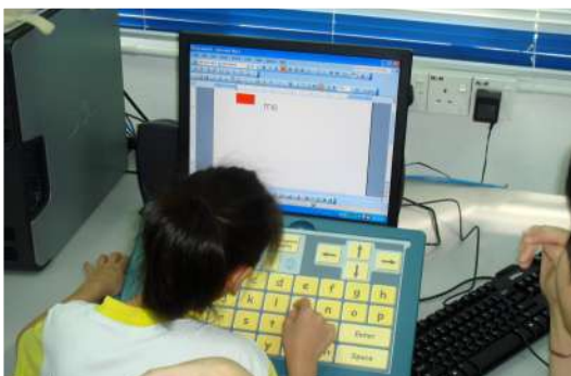
Jeanette is using Intellikeys, a programmable alternative keyboard to complete her work.
