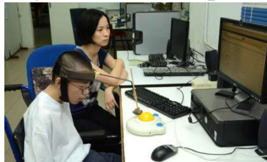
Chee Keong is using the headpointer to control the BIGTrack mouse
