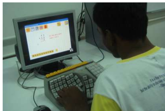
Fredrick accessing the computer with Maltron Single Handed Keyboard
