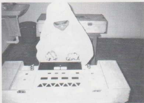
Julia is picking a 25mm steel ball from chute and placing it into the aperture. This is to test a person's ability to perform simple motions such as reach, grasp and release.
